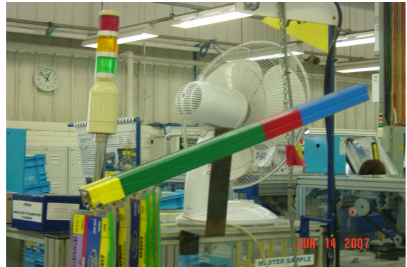
This example of Visual Control shows that the amount of work waiting is within capacity. As the cards get closer to the red mark this would visually indicate there is a problem with the flow or process and needs attention.
