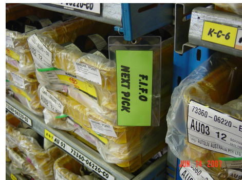
Example Visual Management of Inventory showing First in First Out Control (FIFO)
